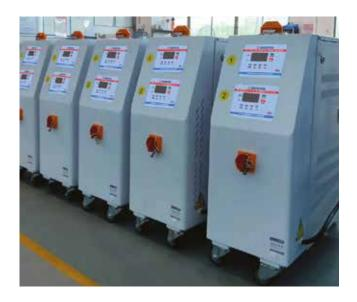
For this reason, MIT thermoregulators (mold conditioners) are often used in plastic injection machines to provide thermal balance.
