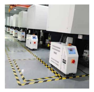
It is essential to use a quality thermoregulator to produce quality products with plastic mold injection. In order for the liquid plastic to remain liquid, it first needs a stable heat balance and then a rapid cooling to freeze. It is nigh impossible to fulfill these two conditions without using a thermoregulator.
